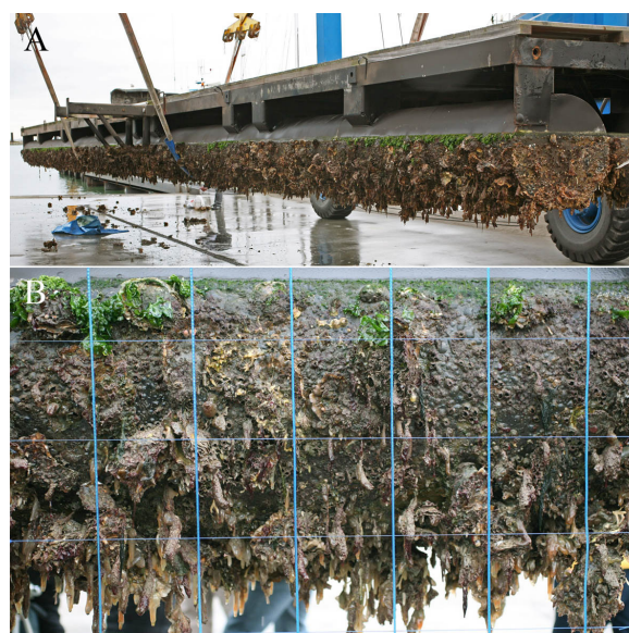
Fig. 12. A heavily fouled floating dock lifted from the water for maintenance. A, Overview; B, Close-up photograph of the fouling. The blue grid lines (used for estimating the fouling cover) form 14x14 cm squares.
